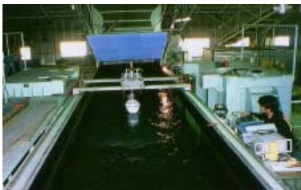
The tank test in IIS of YAJ26 1/10 scale models
