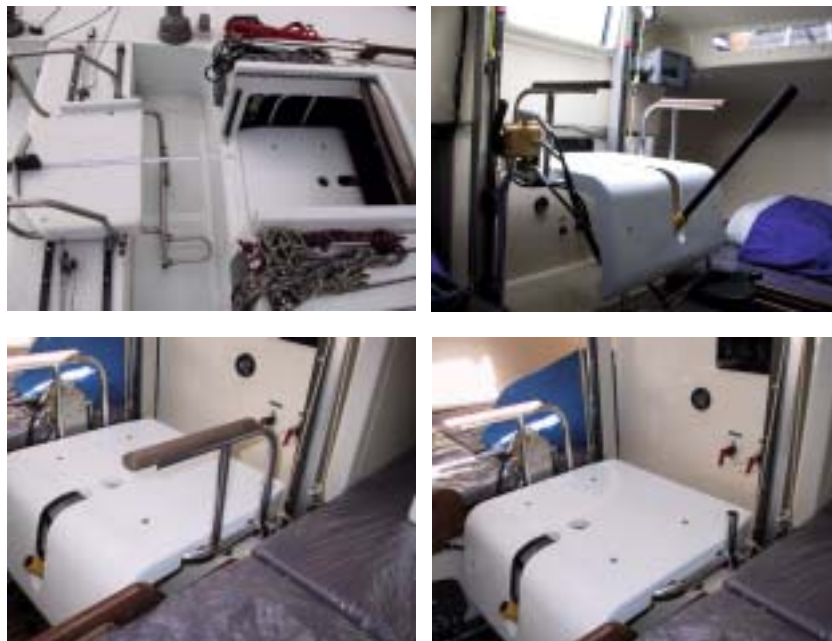
Photos. 6. Hydraulically operated elevator system
