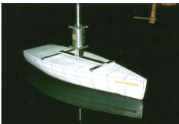
1/10 scale canoe body models for tank test
